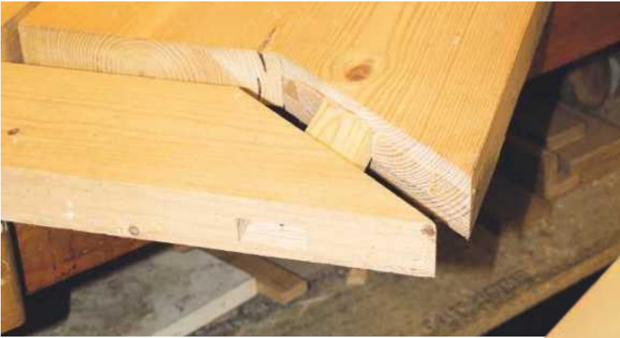
▲ Pic.2 Detail of the through tenon joint often found at table ends. It could also be a stopped tenon so that no end-grain was visible
